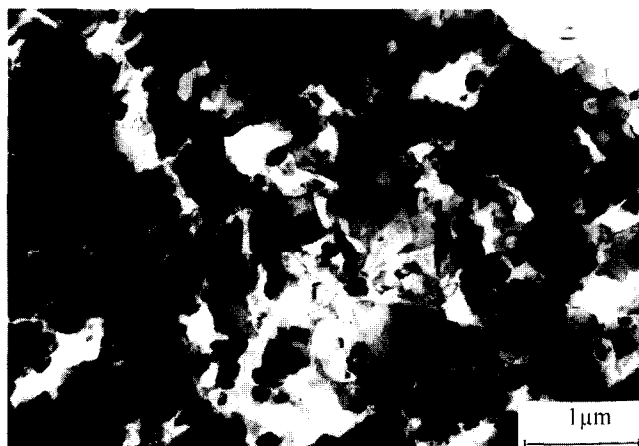
Fig. 3. TEM-micrograph of a porous RBAO material showing a bimodal distribution of the \text{Al}_2\text{O}_3 grain size.
